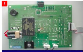
Photograph of MasterMIND monitoring in Current Technology Main Service TVSS unit.
